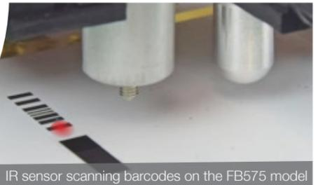
IR sensor scanning barcodes on the FB575 model
